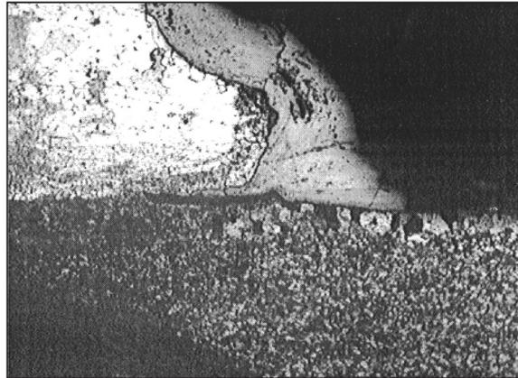
**PHOTOGRAPH 9 MICROSTRUCTURE OF THE WALL OF THE COIL PIPE, LONGITUDINALLY CUT ACROSS A PLACE CLOSE TO THE LEAKY HOLE. GRADUAL WALL THINNING OF THE COIL, GRAIN GROWTH ON THE COIL OUTSIDE SURFACE, THE OUTSIDE FIN AND THE SCALE ON THE OUTSIDE FIN, ALL CAN BE SEEN. (50X)**
