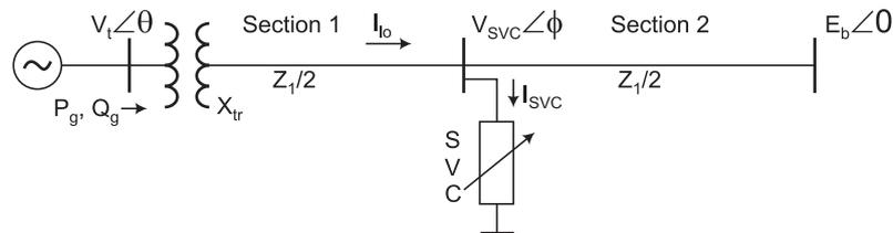
**FIG. 1 SMIB POWER SYSTEM MODEL WITH SVC AT MIDDLE OF THE LINE**
