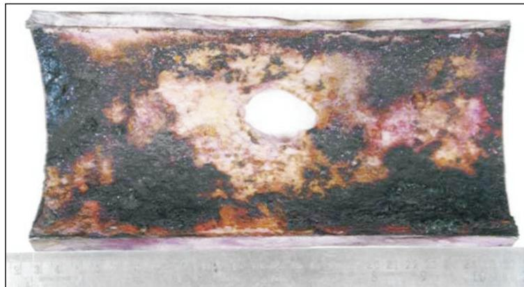
**PHOTOGRAPH 1 THE INSIDE SURFACE OF THE RADIANT COIL NEAR THE LEAKED AREA**
