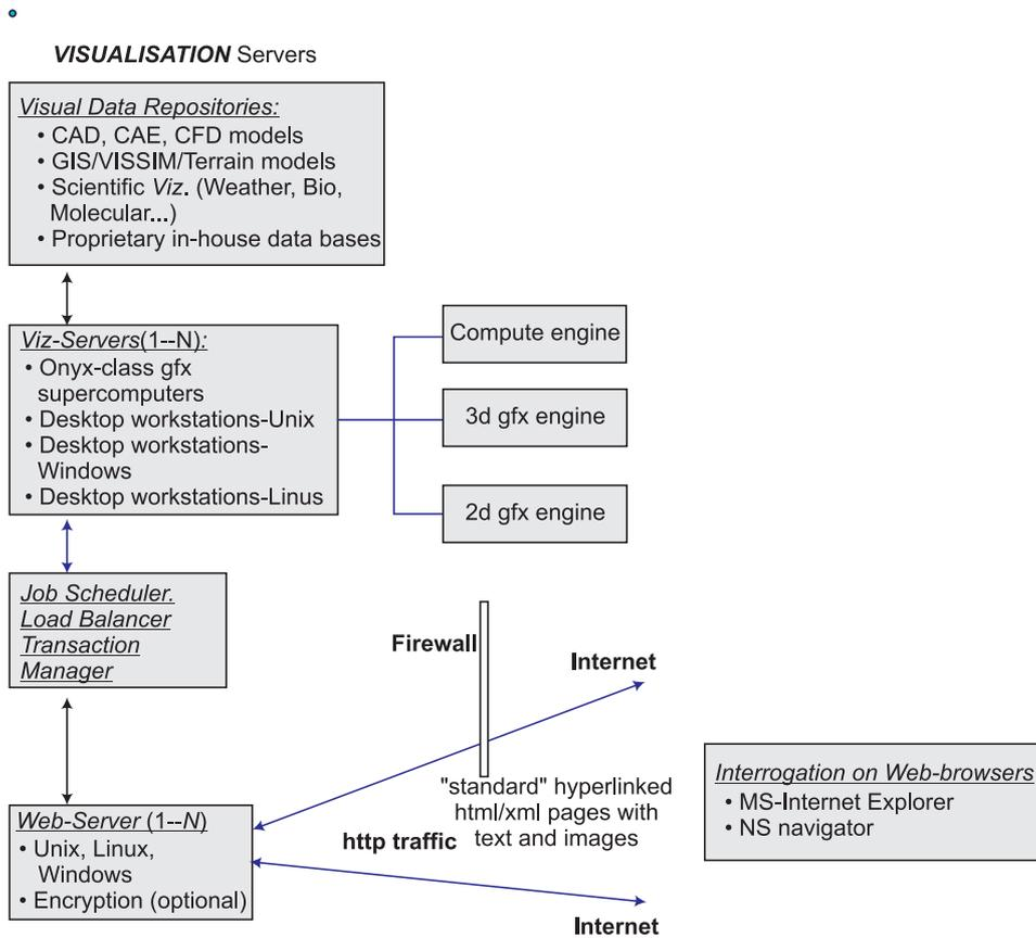
**FIG. 9 VISUALIZATION SERVERS WITH THREE TIER ARCHITECTURE**
