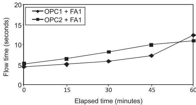
(b) Variation of funnel flow time with elapsed time for mixes with (OPC1 + FA1) and (OPC2 + FA1)
