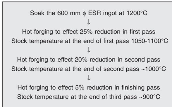
**FIG. 2(a) MODIFIED FORGING SCHEDULE (PHASE 2)**
