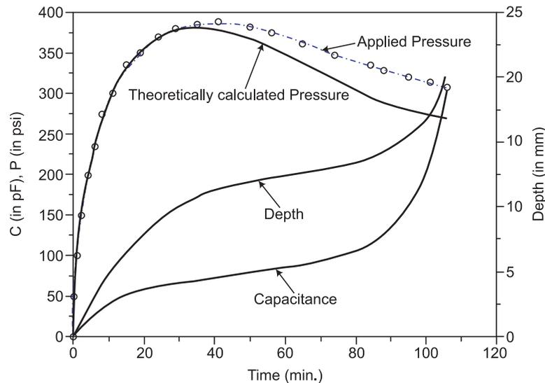
**FIG. 6 PLOTS SHOWING THE VARIATIONS IN CAPACITANCE DEPTH, THEORETICAL PRESSURE AND ACTUALLY APPLIED PRESSURE WITH TIME**
