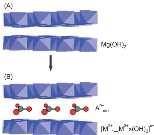
FIG. 5 CRYSTL STRUCUTRE OF BRUCITE (A) AND LDH(B) (REF 6)
