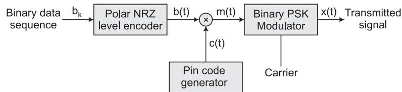
**FIG. 2. DIRECT SEQUENCE SPREAD SPECTRUM COHERENT PSK TRANSMITTER**
