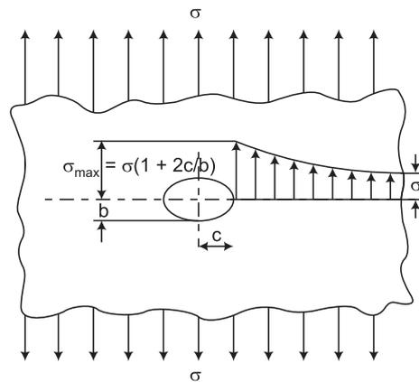
FIG. 2 ELLIPTICAL HOLE IN AN INFINITE PLATE
