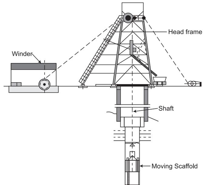
**FIG. 5 HEAD FRAME AND MOVING SCAFFOLD**
