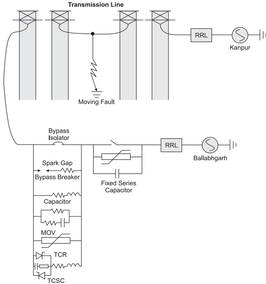
**FIG. 2 SIMPLIFIED REPRESENTATION OF THE LINE, FSC AND TCSC RTDS MODELS**
