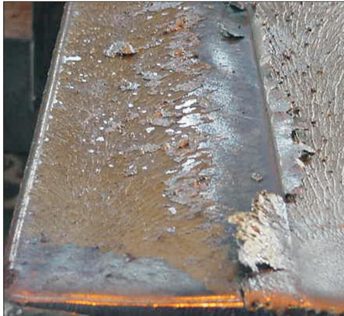
**FIG. 4B DIFFICULT REMOVAL OF STICKY SCALES FROM SLAB SURFACE**
