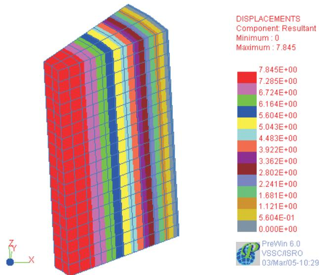
**FIG. 7(c) RESULTANT DISPLACEMENT CONTOUR UNDER GRAVITY LOAD**
