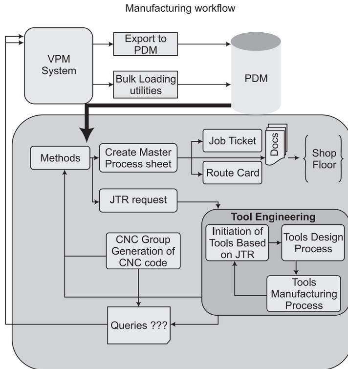
**FIG. 5 MANUFACTURING WORKFLOW**
