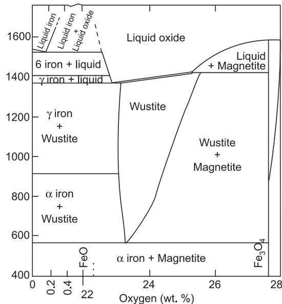
FIG. 2 IRON-OXYGEN PHASE DIAGRAM
