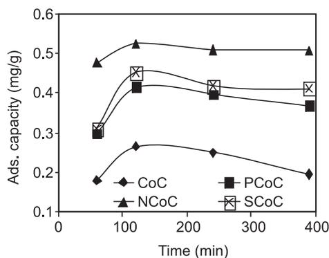
**FIG. 2 DEFLUORIDATION CAPACITIES OF RAW AND ACID TREATED COCONUT COIR (V: 50 ML; C<sub>0</sub>: 8.2 MG/L; W: 0.2 G)**
