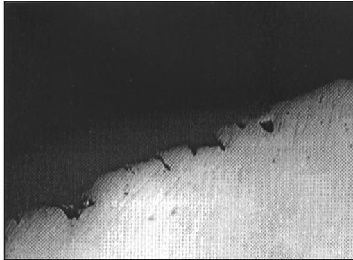
**PHOTOGRAPH 2 LOCALIZED DEEP PITS ON THE INSIDE SURFACE OF ALCOHOL VAPOR SUPERHEATER TUBES. AS POLISHED (200X)**
