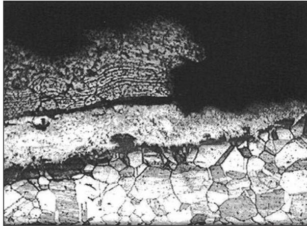
**PHOTOGRAPH 3 PHOTOMICROGRAPH OF A CROSS SECTION ACROSS A LEAKED HOLE NEAR THE INSIDE SURFACE OF THE RADIANT COIL. (50X)**
