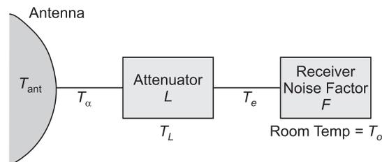
FIG. 1 ANTENNA CONNECTED TO THE RECEIVER BY A CABLE OF LOSS  $L$
