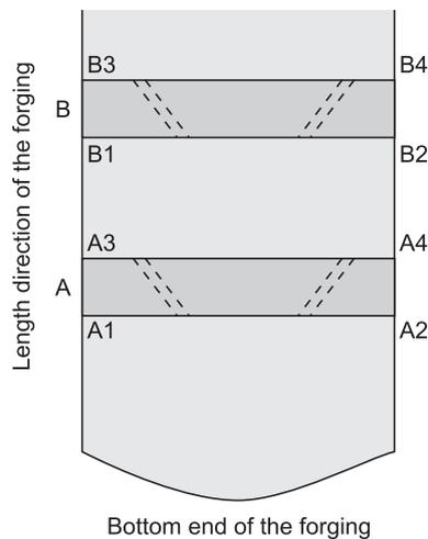
FIG. 5 SCHEMATIC OF FRECKLE-LIKE DEFECTS IN ESR QUALITY FORGINGS
