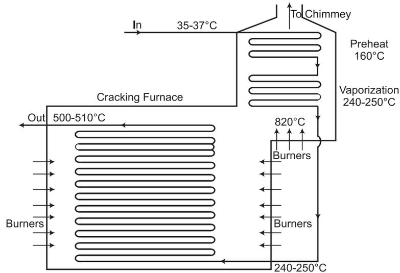
**FIG. 1 FURNACE COIL FOR CRACKING ORGANIC CHLORIDE**
