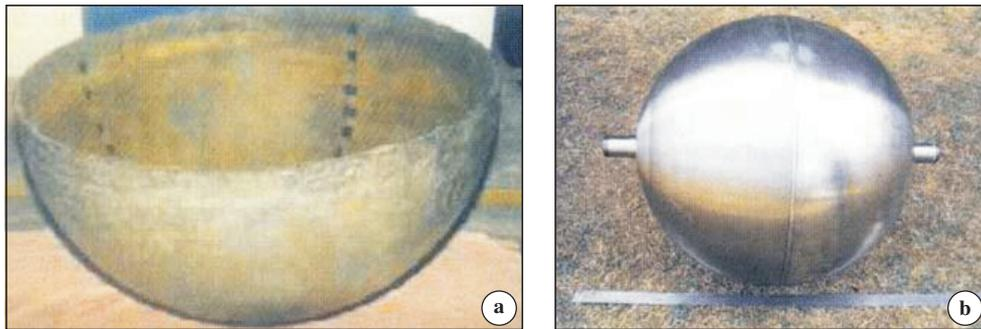
**FIG. 7 (a) HEMISPHERICAL DOME IN STA CONDITION (1200 MM DIA).
