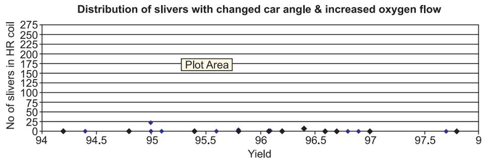
**FIG. 9 SLIVER DISTRIBUTION AS A MEASURE OF THE EFFECTIVENESS OF IMPROVED SCARFING**
