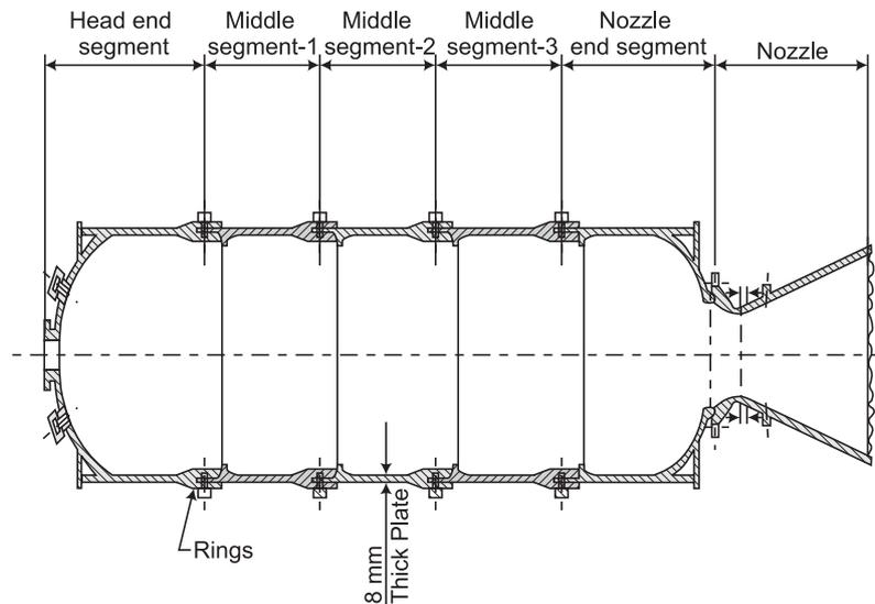
**FIG. 2 SCHEMATIC DIAGRAM OF PSLV FIRST STAGE MOTOR CASE**
