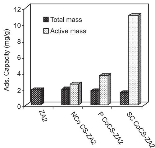
**FIG. 4 DEFLUORIDATION CAPACITIES OF UNSUPPORTED AND COCONUT COIR SUPPORTED LDH ALONG WITH THE ADSORPTION CAPACITY OF THE ACTIVE MASS (CALCULATED BASED ON MATERIAL BALANCE) (V: 50 ML;  $C_0$ : 8.1 MG/L; W: 0.2 G; T: 360 MIN)**
