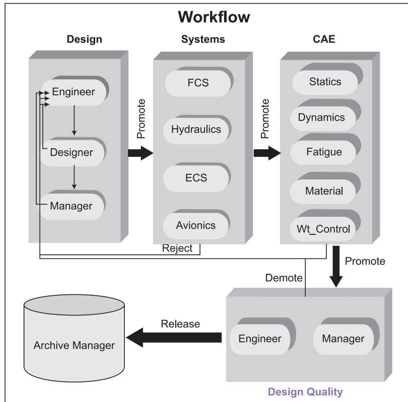
FIG. 4 DESIGN WORKFLOW FOR TYPICAL AIRCRAFT DESIGN
