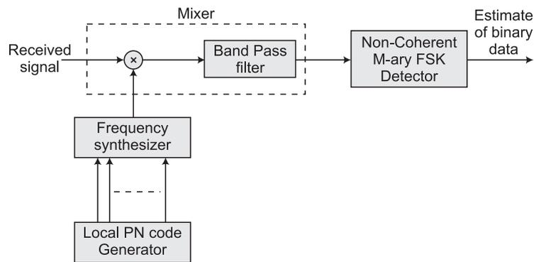
**FIG. 5 FREQUENCY-HOP SPREAD SPECTRUM M-ARY FSK RECEIVER**
