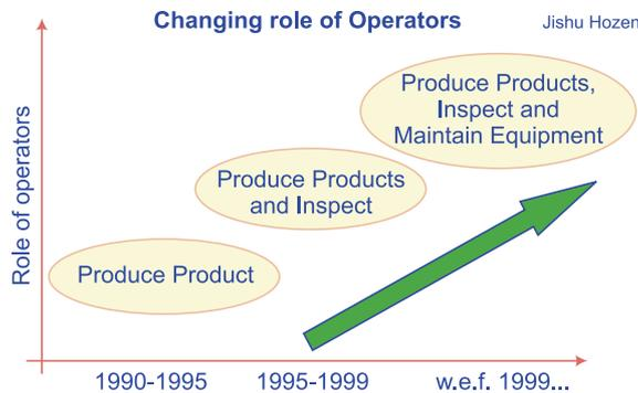
The Japanese Jishu Hozen concept in Total Predictive Maintenance (TPM) gradually leads to a situation of autonomous maintenance of equipment, leading to increased availability, improved quality and superior performance.
