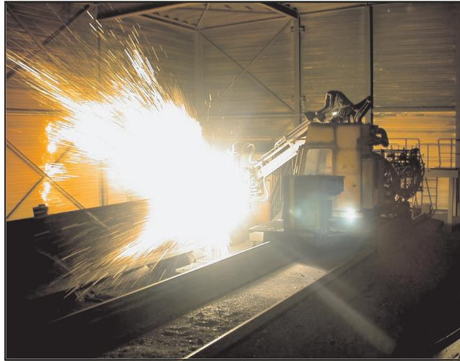
**FIG. 3 SCARFING OF SLABS BY AUTOMATIC SCARFER**
