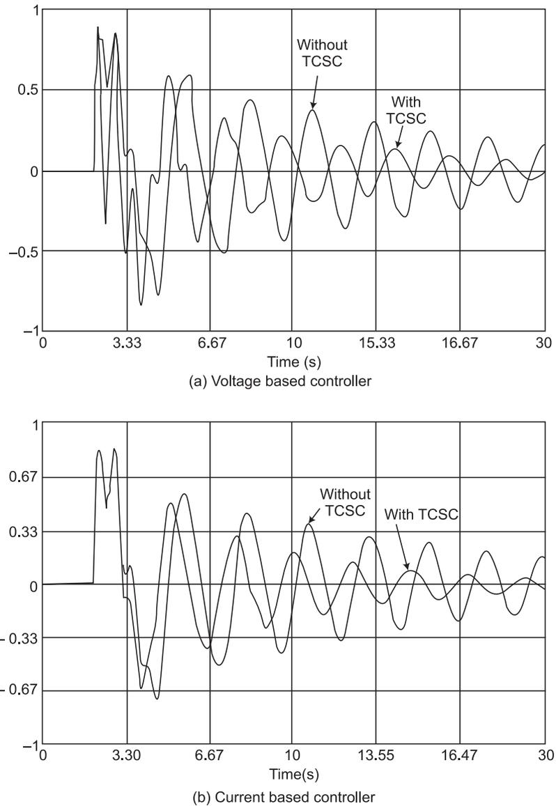
**FIG. 9 DAMPING OF OUTAGE OF HVDC LINE ON RTDS**
