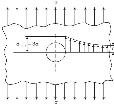
FIG. 1 CIRCULAR HOLE IN AN INFINITE PLATE
