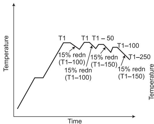
**FIG. 1(b) SCHEMATIC OF HOT FORGING SCHEDULE FOLLOWED IN THE BEGINNING (PHASE 1)**
