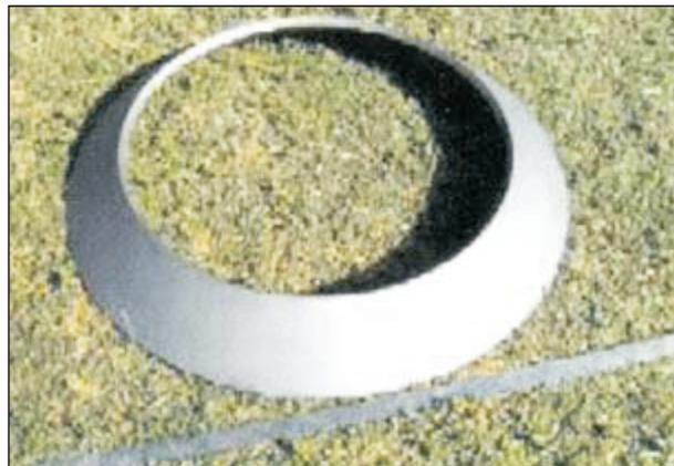
**FIG. 8 SEAMLESS CONICAL COMPONENT DEVELOPED THROUGH PLATE-FORMING ROUTE (850 MM MAX. DIA., 45 DEGREE CONE ANGLE)**
