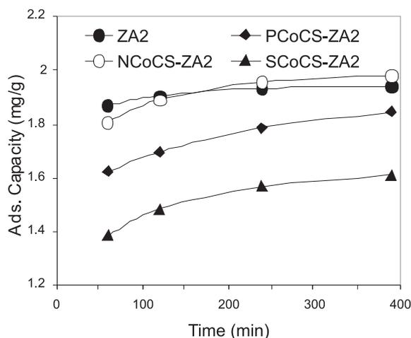
**FIG. 3 A COMPARISON OF THE DEFLUORIDATION CAPACITIES OF THE UNSUPPORTED AND COCONUT COIR SUPPORTED ZN/AL LDH (V: 50 ML; C0: 8.1 MG/L; W: 0.2 G)**
