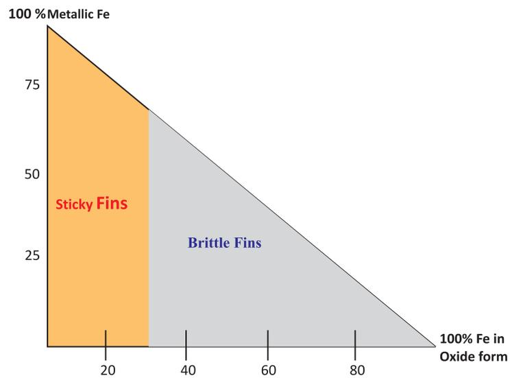
**FIG. 5 PERCENTAGE OF METALLIC FE & FE IN OXIDE FORM AFFECTING FIN QUALITY**
