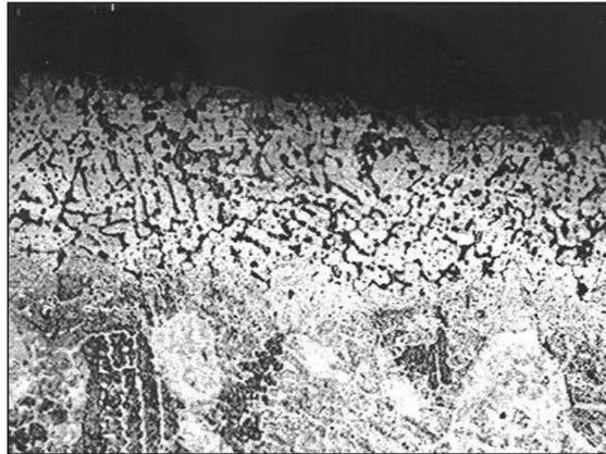
**PHOTOGRAPH 7 MICROSTRUCTURE ACROSS THE WALL OF THE BOWED TUBE AT THE OUTSIDE SURFACE NEAR THE BOTTOM-MOST POSITION (100X)**
