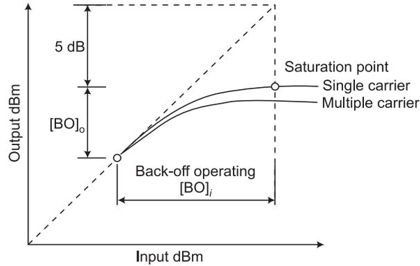
**FIG. 2 OUTPUT POWER SATURATION OF SATELLITE TWTA**
