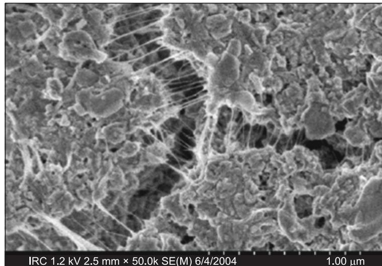
**FIG. 3 CRACK BRIDGING BY CNT BUNDLES WITH CEMENT MATRIX(REF 3)**
