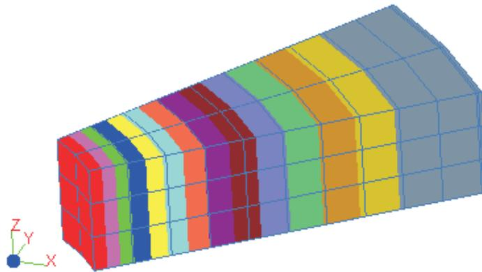
**FIG. 7(b) RESULTANT DISPLACEMENT CONTOUR UNDER THERMAL LOAD**
