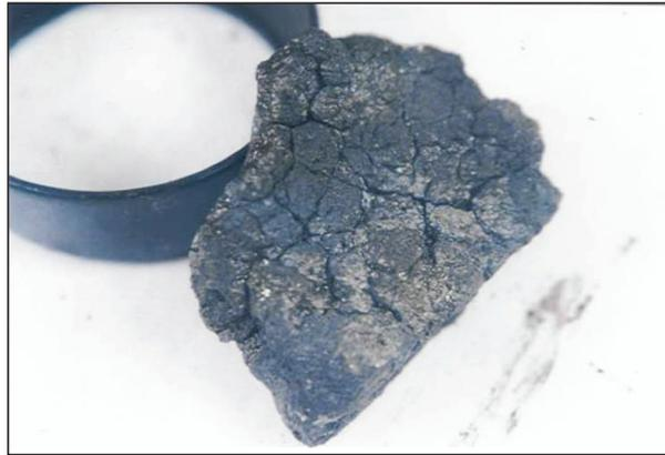
**PHOTOGRAPH 2 A SAMPLE OF A COKE LUMP COLLECTED FROM THE INSIDE SURFACE OF THE RADIANT COIL**
