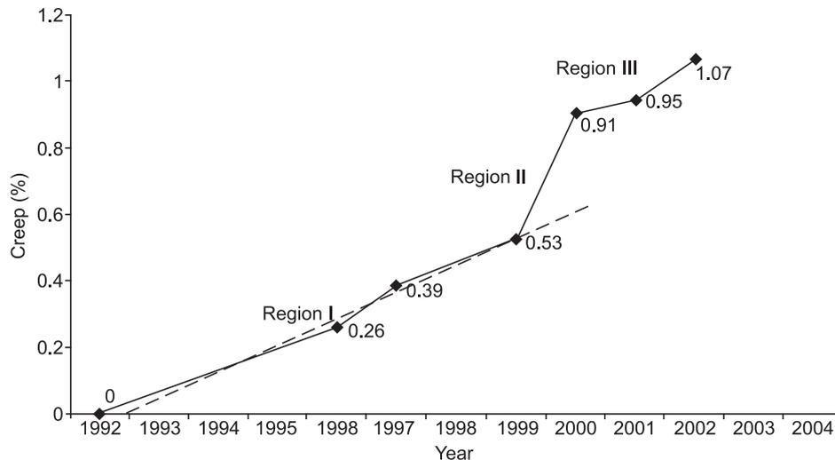
**FIG. 3 PROGRESS OF CREEP OF THE BOWED TUBE**
