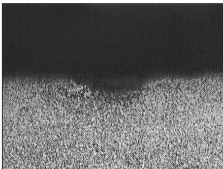
**PHOTOGRAPH 1 MICROSTRUCTURE ACROSS ONE OF THE CORRODED PITS IN THE TUBE SAMPLE. LOCALIZATION OF ATTACK WITHOUT ANY EFFECT ON THE NEARBY OUTSIDE SURFACE OF THE TUBE. (50X)**
