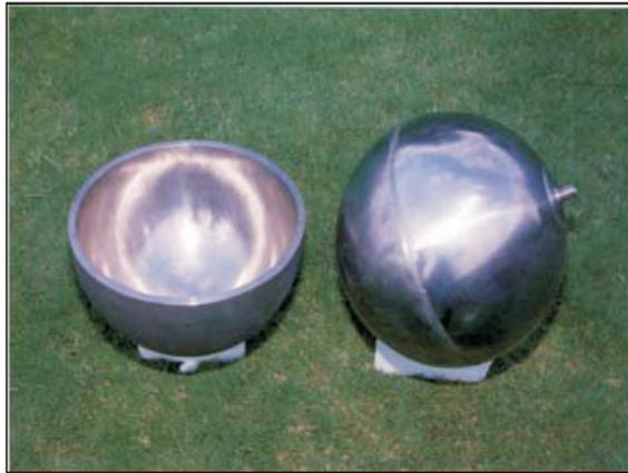
**FIG. 6 SUPERPLASTICALLY FORMED HEMISPHERE AND ELECTRON BEAM WELDED AIR BOTTLE MADE OF ELI GRADE Ti-6Al-4V**
