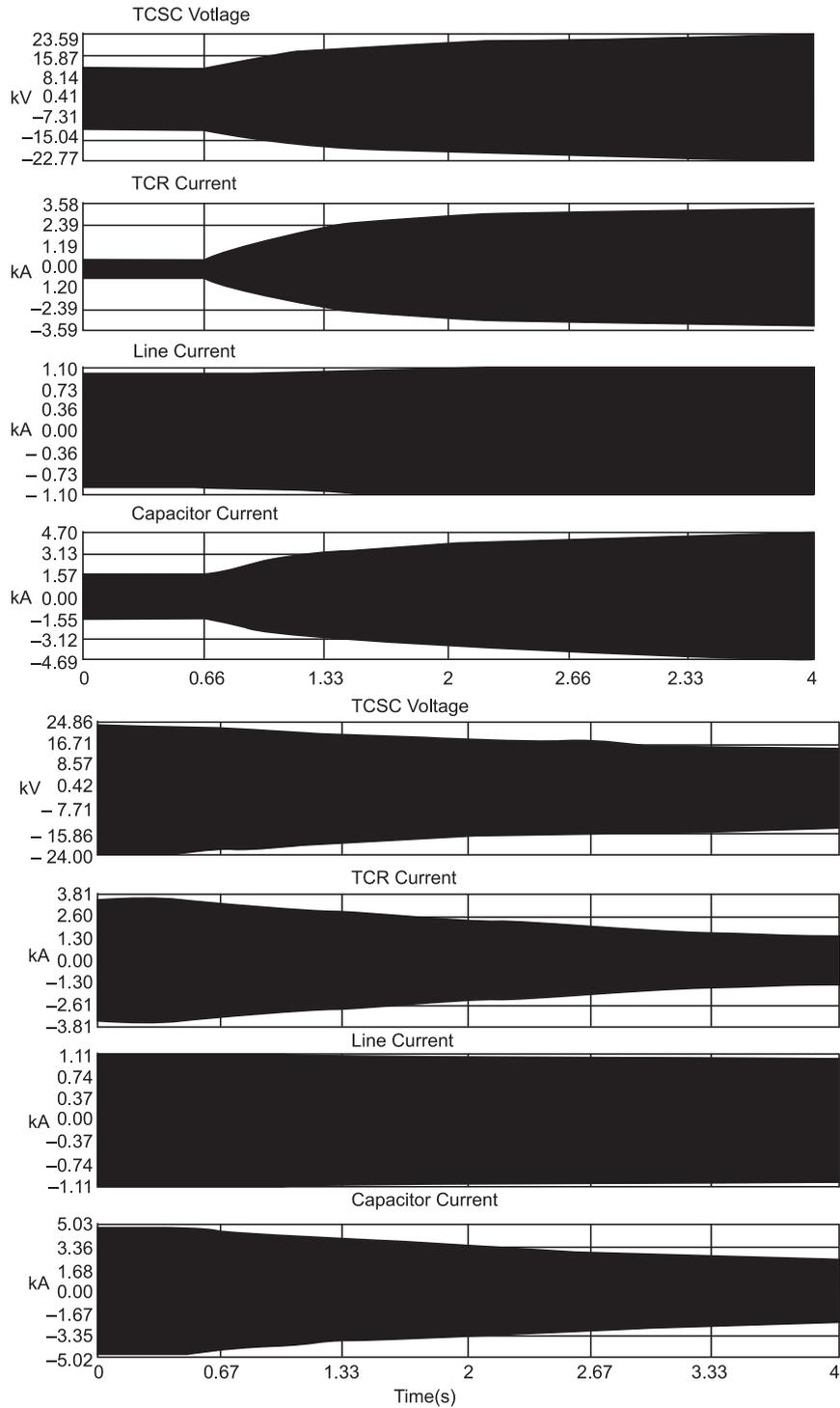
FIG. 6 STEP CHANGE (INCREASE/DECREASE) IN LINE CURRENT
