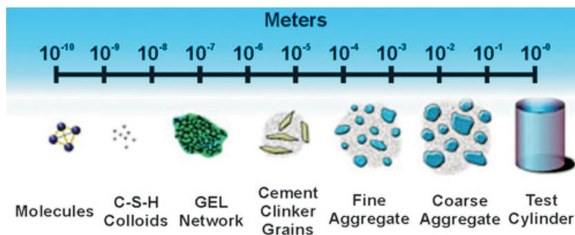
FIG. 1 SCALES OF VARIOUS CONSTITUENTS OF CONCRETE (REF 1)
