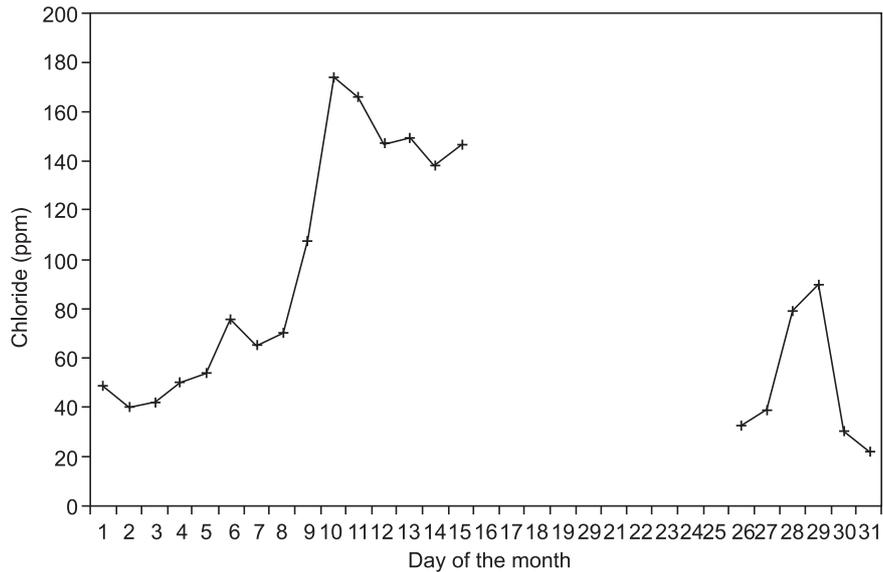
**FIG. 1 VARIATION OF DAILY AVERAGE CHLORIDE LEVEL IN THE BLOW-DOWN WATER IN A MONTH WHEN LEAKAGE OCCURRED**
