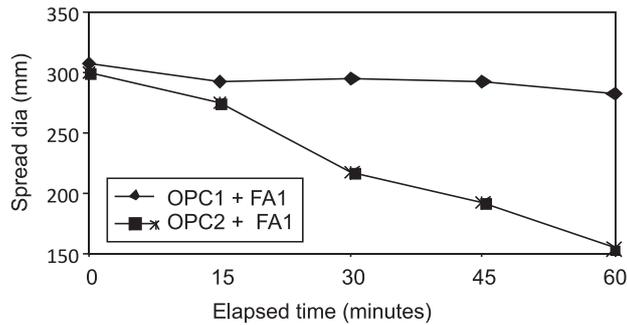
(a) Variation of spread diameter with elapsed time for mixes with (OPC1 + FA1) and (OPC2 + FA1)
