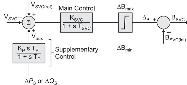
**FIG. 2 BLOCK DIAGRAM OF SVC WITH AUXILIARY CONTROL**
