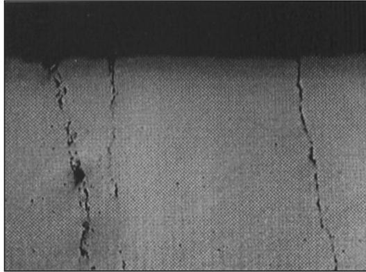
**PHOTOGRAPH 4 CHLORIDE STRESS CORROSION CRACKS INITIATING ON MULTIPLE PLACES ON LOCALIZED PITS ON THE INSIDE SURFACE OF ALCOHOL VAPOR SUPERHEATER TUBE. (50X)**
