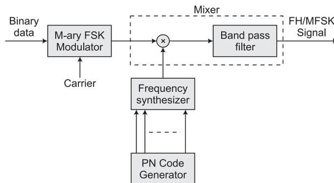
**FIG. 4 FREQUENCY-HOP SPREAD SPECTRUM M-ARY FSK TRANSMITTER**
