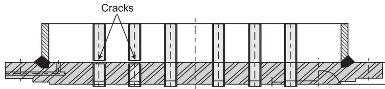
**FIG. 3 A SKETCH OF THE ELEVATION OF THE BOTTOM PORTION OF THE ALCOHOL VAPOR SUPERHEATER. SHOWS CIRCUMFERENTIAL CRACKS ON THE TUBES JUST ABOVE THE TOP SURFACE OF THE BOTTOM TUBE-SHEET**
