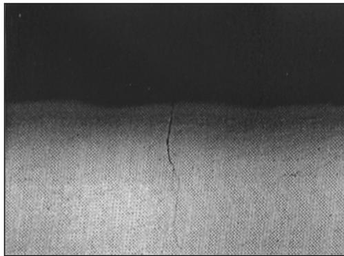
**PHOTOGRAPH 3 CHLORIDE STRESS CORROSION CRACK INITIATING ON SMOOTH PORTION OF THE INSIDE SURFACE OF THE ALCOHOL VAPOR SUPERHEATER. AS POLISHED (100X)**
