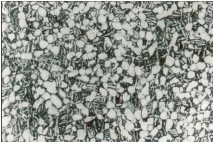
**FIG. 4(b) MICROSTRUCTURE OBTAINED BY MODIFIED PROCESSING ROUTE WITH ANNEALING IN THE  $\alpha + \beta$  PHASE FIELD AT 950°C**
