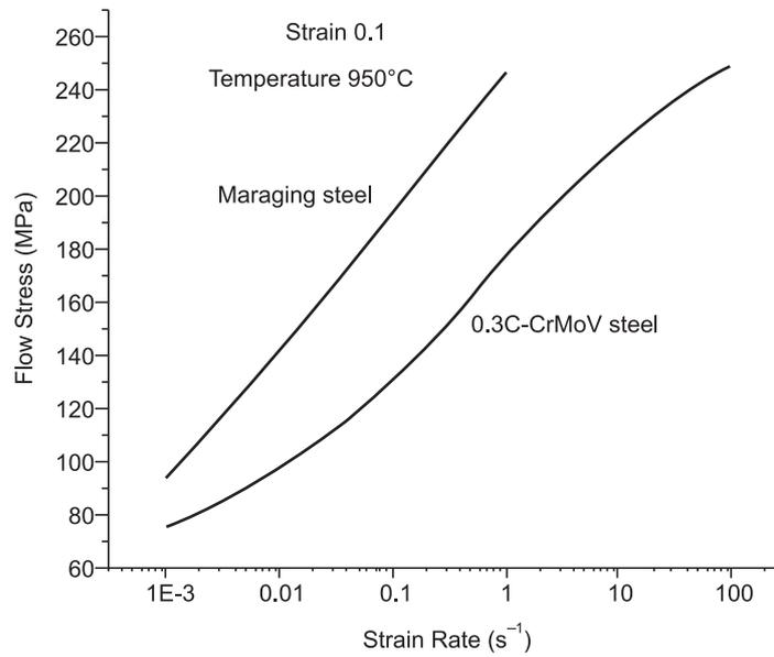
**FIG. 5 VARIATION OF FLOW STRESS WITH CHANGE IN STRAIN RATE**
