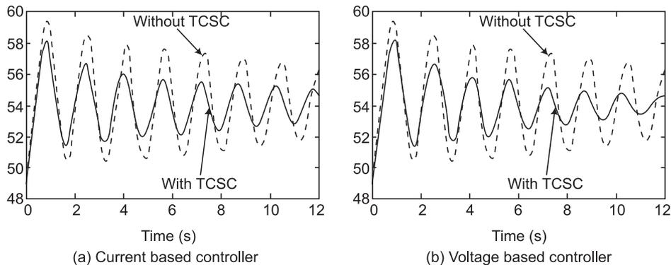
**FIG. 8 DAMPING OF OUTAGE OF HVDC LINE ON MATLAB**
