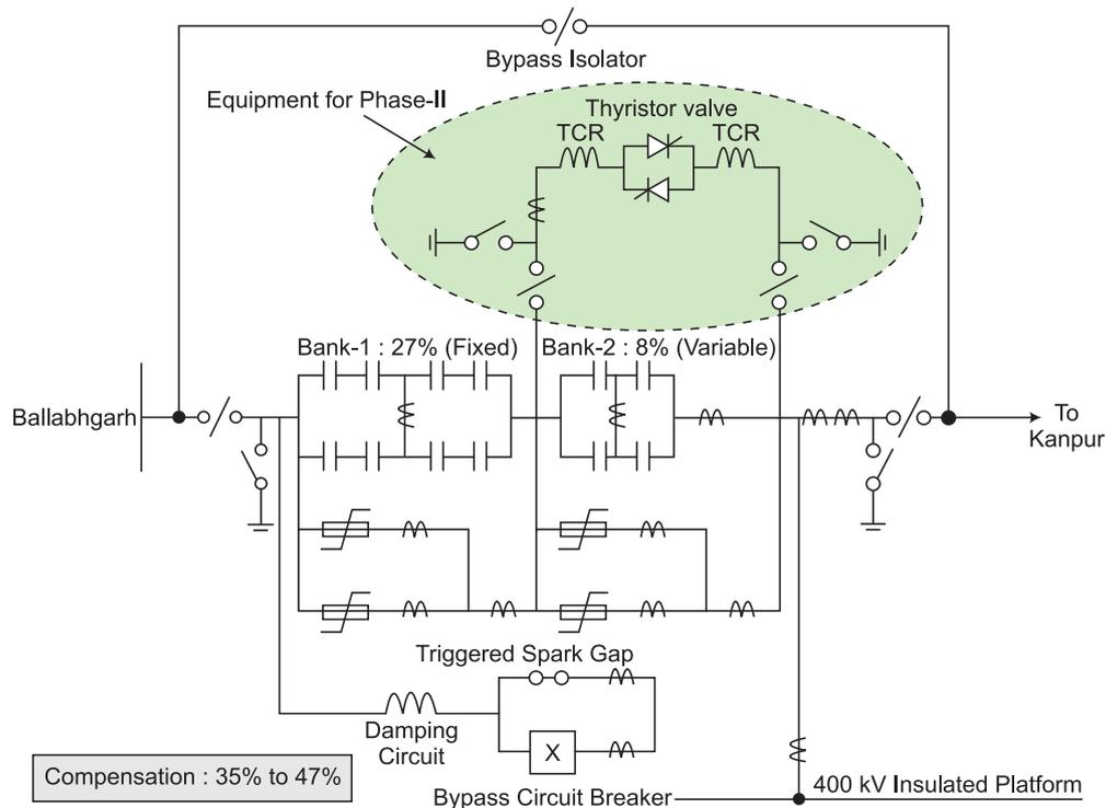
**FIG. 1 SINGLE LINE DIAGRAM OF THE TCSC SCHEME**
