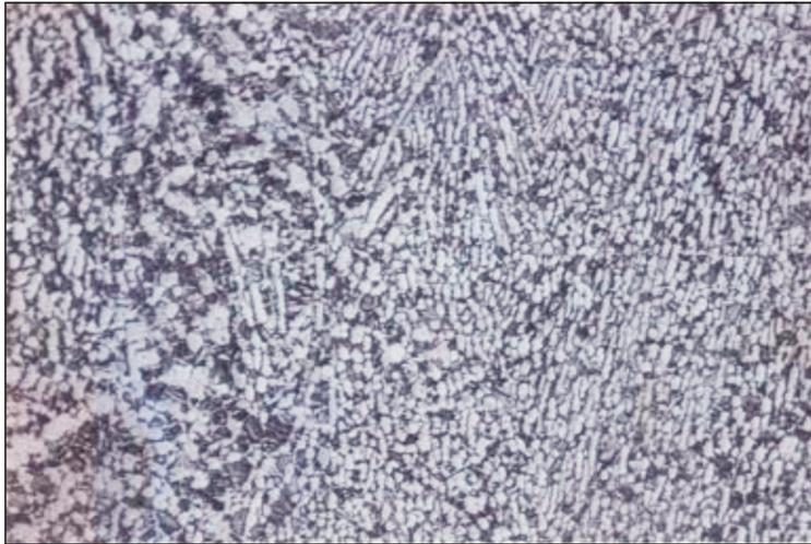
**FIG. 4(a) MICROSTRUCTURE OBTAINED BY MODIFIED PROCESSING ROUTE WITH ANNEALING IN THE  $\alpha + \beta$  PHASE FIELD AT 700°C**
