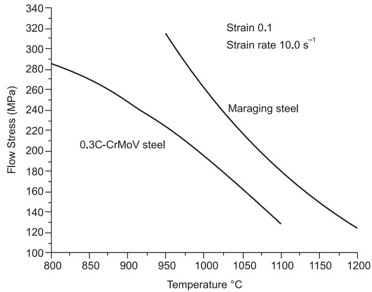
**FIG. 4 VARIATION OF FLOW STRESS AS A FUNCTION OF TEMPERATURE AT A STRAIN LEVEL OF 0.1 AT A STRAIN RATE OF 10.0/SEC**
