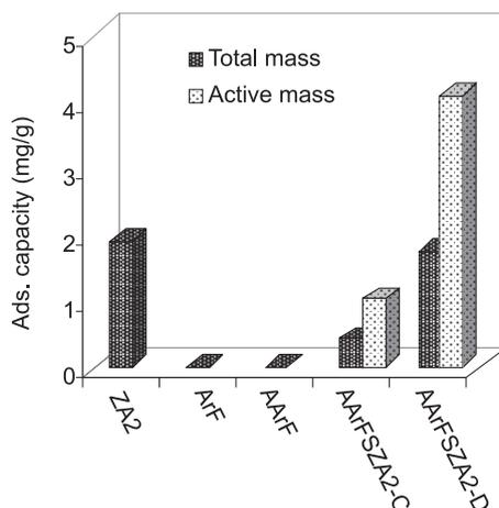
**FIG. 1 DEFLUORIDATION CAPACITIES OF SUPPORTED LDH, ACTIVE LDH PRESENT ON THE SUPPORT AND ARECA NUT FIBER (V: 50 ML; C<sub>0</sub>: 8.1 MG/L; W: 0.2 G; T: 240 MIN)**
