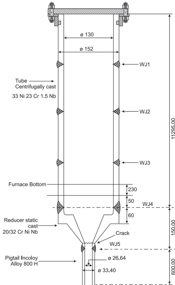
**FIG. 2 PRIMARY REFORMER TUBE WITH REDUCER**
