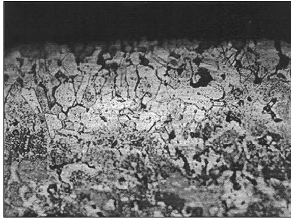
**PHOTOGRAPH 9 MICROSTRUCTURE ACROSS THE WALL OF THE BOWED TUBE AT THE OUTSIDE SURFACE AT A PLACE WHERE MAXIMUM ULTRASONIC ATTENUATION WAS 22% (200X)**
