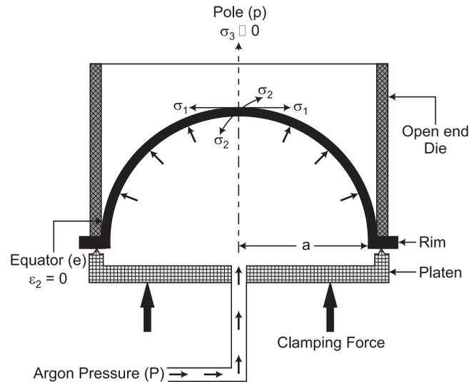
**FIG. 1 SCHEMATIC GAS PRESSURE SUPERPLASTIC FORMING OF HEMISPHERE**
