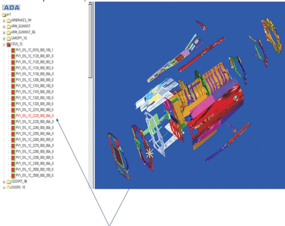
**FIG. 10 TREE BASE PRODUCT STRUCTURE FOR WEB BROWSER USING VISUALIZATION SERVER**
