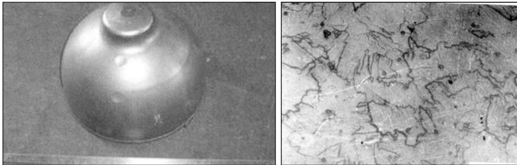
**FIG. 9 Ti5Al2.5Sn ELI ALLOY HEMISPHERICAL FORGINGS FOR HIGH PRESSURE GAS BOTTLES FOR LIQUID HYDROGEN ENVIRONMENT WITH SINGLE PHASE  $\alpha$  MICROSTRUCTURE**
