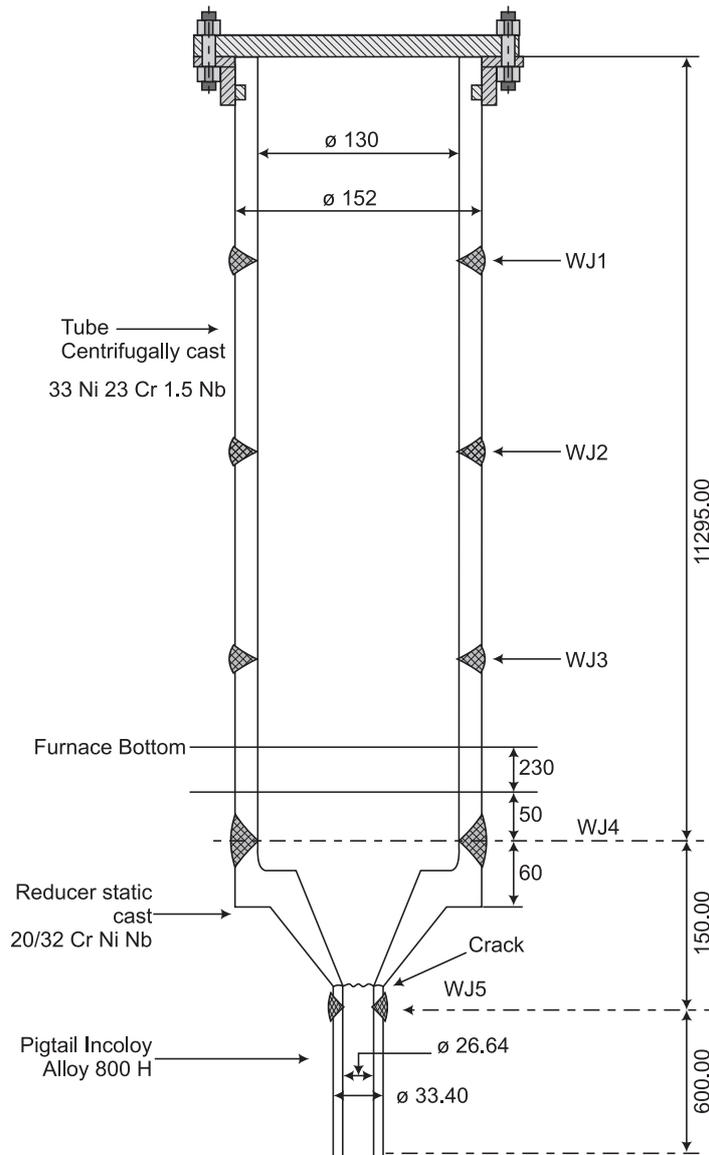
**FIG. 2 PRIMARY REFORMER TUBE WITH REDUCER**
