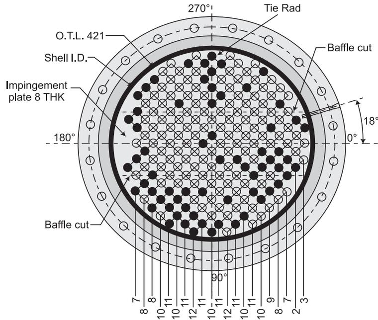
**FIG. 2 CROSS-SECTION OF THE ALCOHOL VAPOR SUPERHEATER WITH LEAKED TUBES SHOWN AS FULL BLACK CIRCLES**
