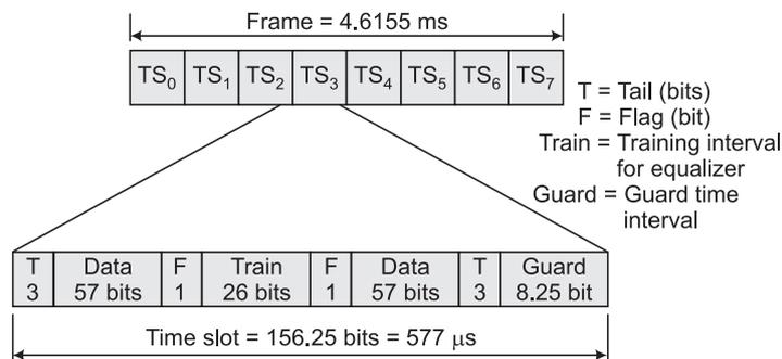
**FIG. 6 FRAME STRUCTURE OF THE GSM WIRELESS COMMUNICATION SYSTEM**
