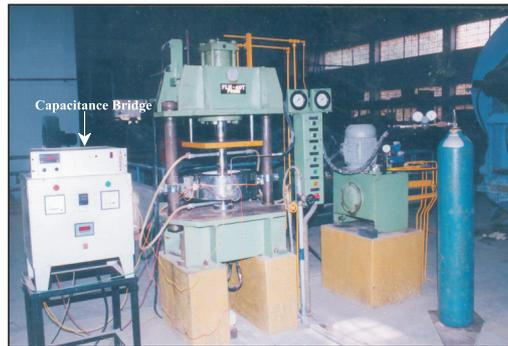
**FIG. 4 SUPERPLASTIC BLOW FORMING SET-UP ALONG WITH THE CAPACITANCE BRIDGE**
