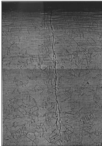
**PHOTOGRAPH 5 COMPOSITE PHOTOMICROGRAPH OF A CHLORIDE STRESS CORROSION CRACK INITIATING ON THE INSIDE SURFACE AND PROPAGATING TOWARDS THE OUTSIDE SURFACE, TRANSGRANULAR WITH BRANCHING (100X)**
