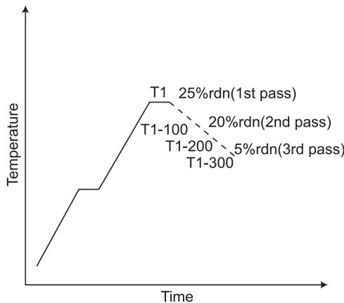
**FIG. 2(b) SCHEMATIC OF HOT FORGING SCHEDULE FOLLOWED AFTER INCORPORATING MAJOR CHANGES**
