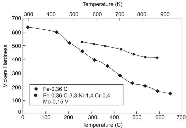
**FIG. 4 RELATIVE TEMPERING BEHAVIOR OF A PLAIN CARBON STEEL AND A NICRMOV LOW ALLOY STEEL, BOTH HAVING THE SAME CARBON LEVEL**
