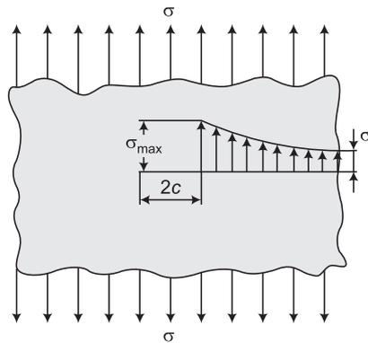
**FIG. 3 CRACK IN AN INFINITE PLATE**
