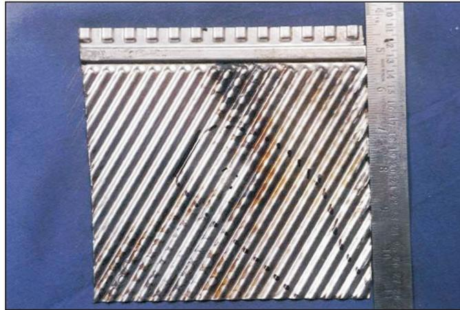
**PHOTOGRAPH 12 COOLING WATER SIDE OF THE AFFECTED PLATE ELEMENTS
