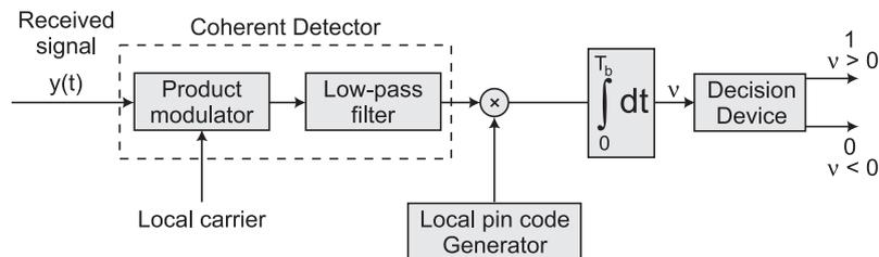
**FIG. 3 DIRECT SEQUENCE SPREAD SPECTRUM COHERENT PSK RECEIVER**
