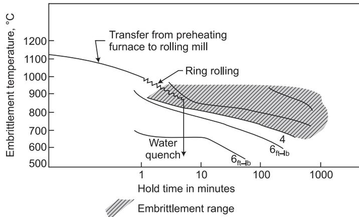
**FIG. 3 SCHEMATIC OF THERMO-MECHANICAL WORKING ATTEMPTED**
