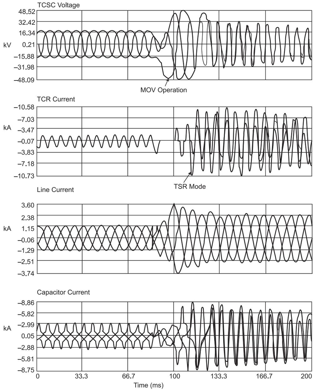
**FIG. 7 THREE PHASE TO GROUND FAULT ON KANPUR-BALLABHGARH TRANSMISSION LINE**
