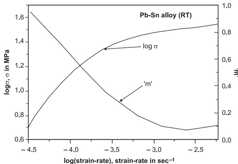
**FIG. 5 PLOTS SHOWING “STRESS VS. STRAIN-RATE” (ON LOG-LOG SCALE) AND “M’ VS. STRAIN-RATE (LOG SCALE)” FOR Pb-Sn ALLOY AT RT**
