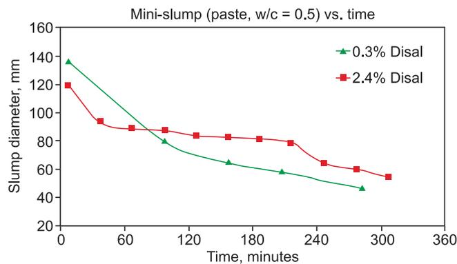
FIG. 6 SLUMP RETENTION WITH LDH TECHNOLOGY (REF 6)
