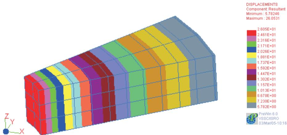
**FIG. 7(a) RESULTANT DISPLACEMENT CONTOUR UNDER PRESSURE LOAD**
